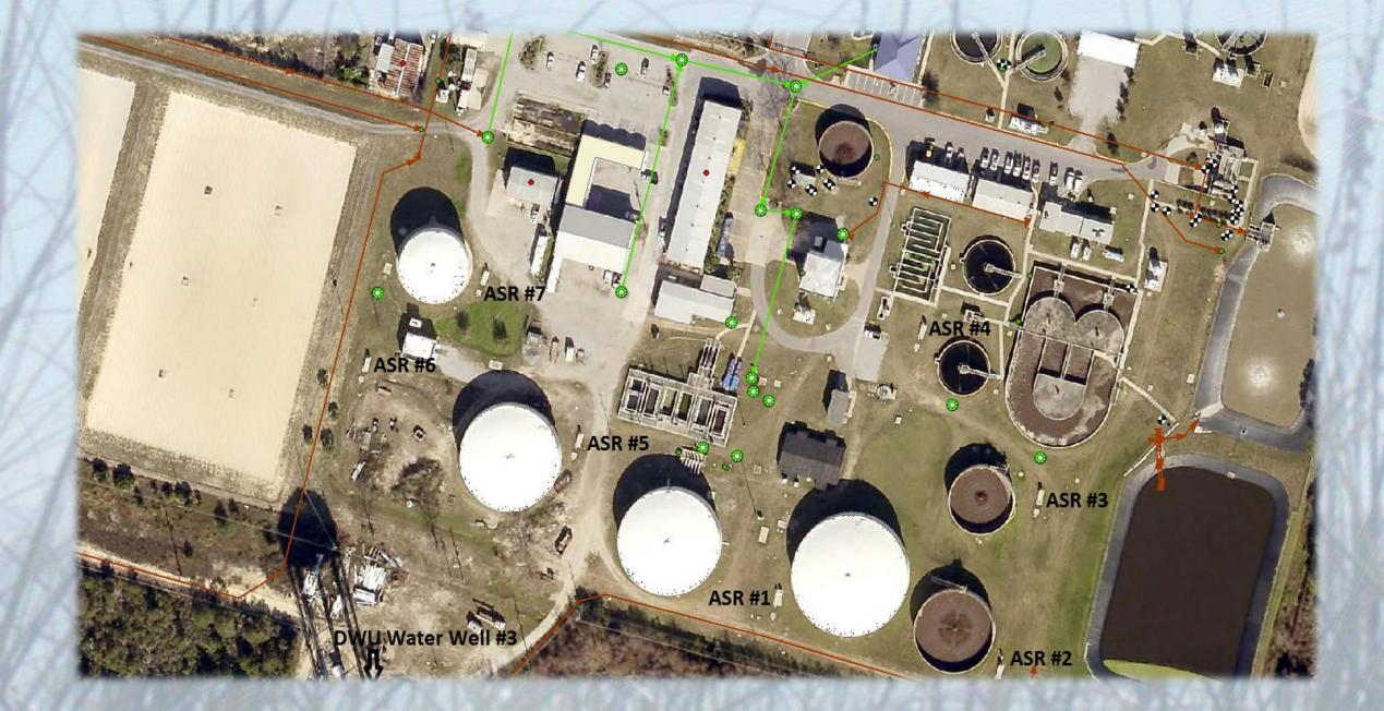
The DWU ASR system is permitted under the FDEP UIC program. All seven wells are located on the Wastewater treatment plant property and are numbered based on the order they were drilled. The data below gives the
